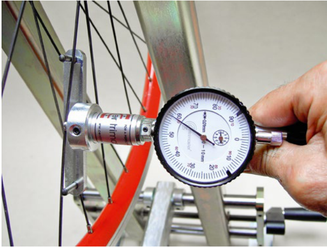
Tensiometer with calibration list, also for bladed spokes
